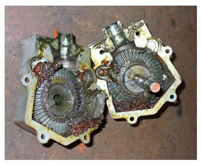
This photo shows the grease found in a Foote 35 from an Early Gear Drive model. The once smooth flowing grease has become clumps and gobs of stiff material that has been driven from the gears into case voids.
